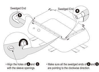
10. Insert the 2U-Shaped Pipe take to the strapes at the bottom of
