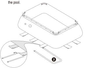
7. Carefully slide the connected Short Tubes **4** into the sleeves on the short sides of the pool.
