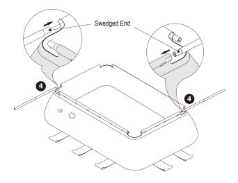
9. Connect the ③ Corner Piece to the takes at 4 Corner. A closed rectanglar pool frame is now frame at the pool top. **NOTE:** The Conner Piece ④ DO NOT have a hole to catch the spring pin. THIS IS NORMAL. Only ④ ⑤ Tubes have holes to catch the spring pin.
