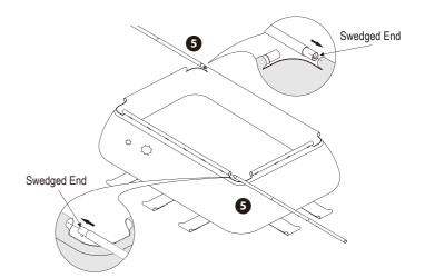
**NOTE:** Refer to the parts list on page 6 for the exact quantity of **S** Tubes. Connect half the total quantity to form the horizontal beams on the long sides of the pool.
